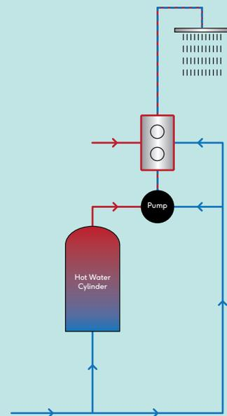
A pump assisted system will deliver water at high pressure and depending on the specifications of the pump fitted LP, MP and HP taps and fittings may be used.
