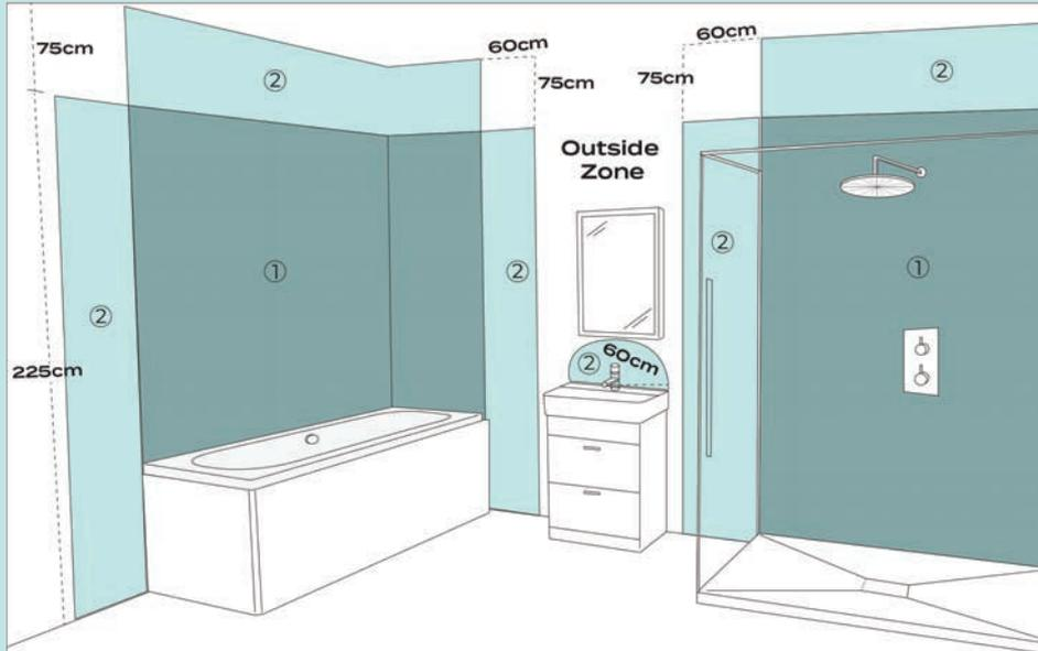
**ZONE 0** – is inside the bath or shower. Any fitting used in this zone must be low voltage (max 12v) and be rated at least voltage (max 12v) and be rated at least IP67 (immersion proof)
