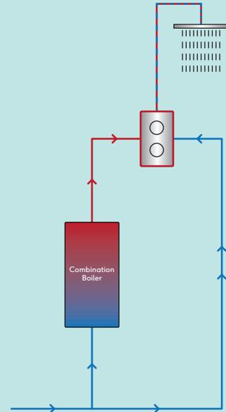
A combination boiler heats water on demand, and although it is fed by mains pressure this is regulated to the speed which the boiler can heat the water.
